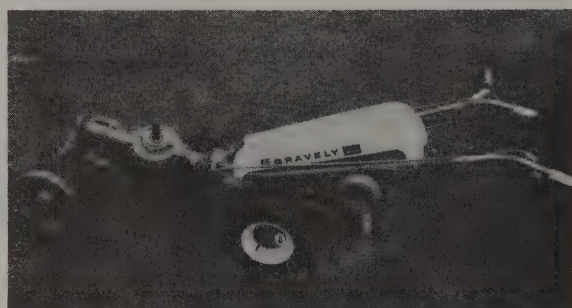
The smallest tractor Gravelly Corporation makes is their 8 hp gas powered "convertible tractor." It has a rotary plough, not a roto-tiller, and sells for $1,200.00. The T-head, 1 cylinder engine is the same design they have been using since the 1920s; 30 years of continuous use is not uncommon. Gravelly is now entirely out of the shredder/composter business. (Gravelly Corporation, Gravelly Lane, Clemmons, North Carolina 27012.) (Also reviewed in CATALOG, p. 55.)
